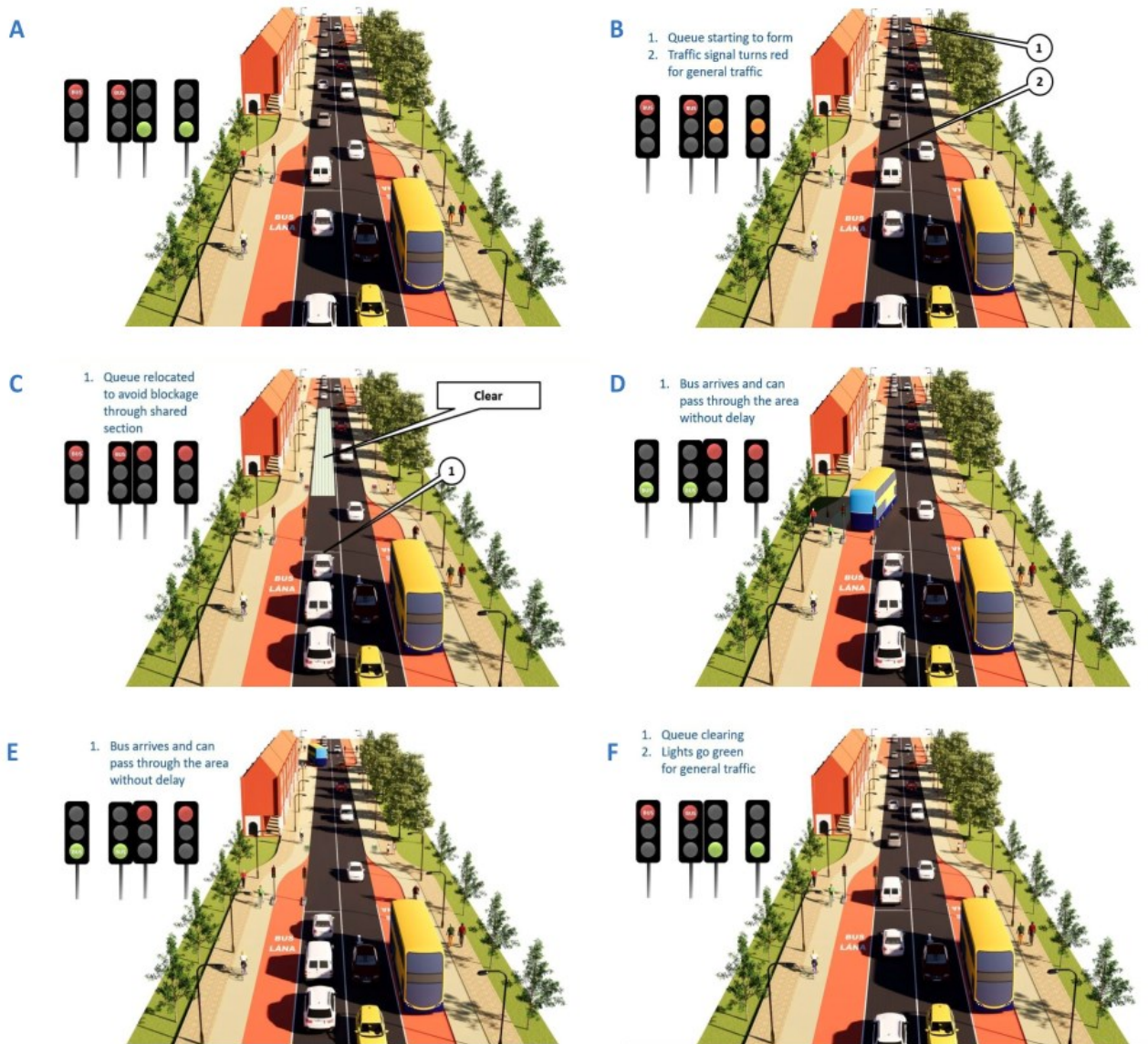
Image 4.10: Signal Controlled Priority Schematic Operation (Source: PDGB)
