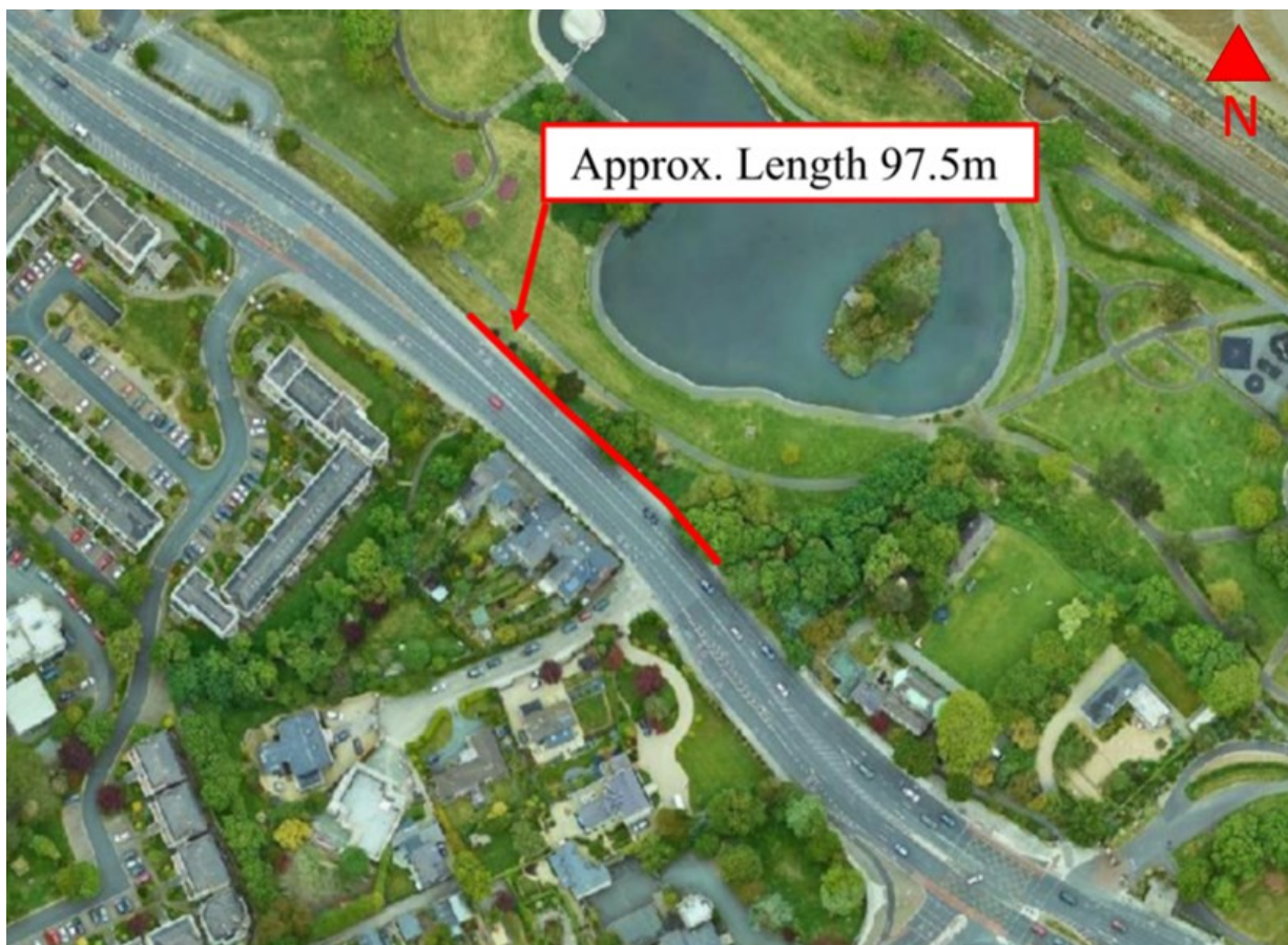
Image 4.18: Location of principal retaining wall
